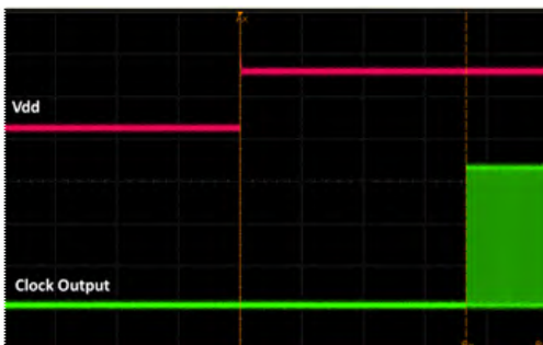
Figure 17. Startup Waveform vs. Vdd
