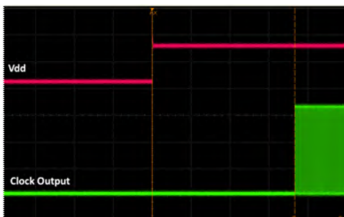
Figure 17. Startup Waveform vs. Vdd
