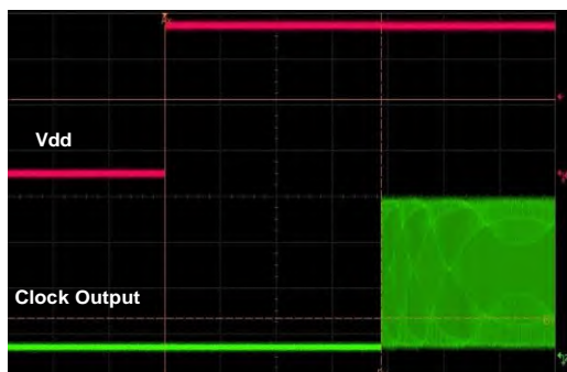
Figure 17. Startup Waveform vs. Vdd
